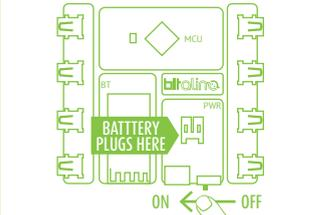
You can easily confirm that the device is turned on, as a white LED will start fading on the Microcontroller (MCU) Block.
